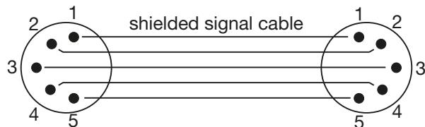
The Sparx10 has 3pin and 5pin XLR connectors for DMX-in and DMX-out. Do not connect more than one data input and one data output on a fixture.
