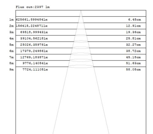
Note: The Curves indicate the illuminated area and the average illumination when the luminaire is at different distance.
