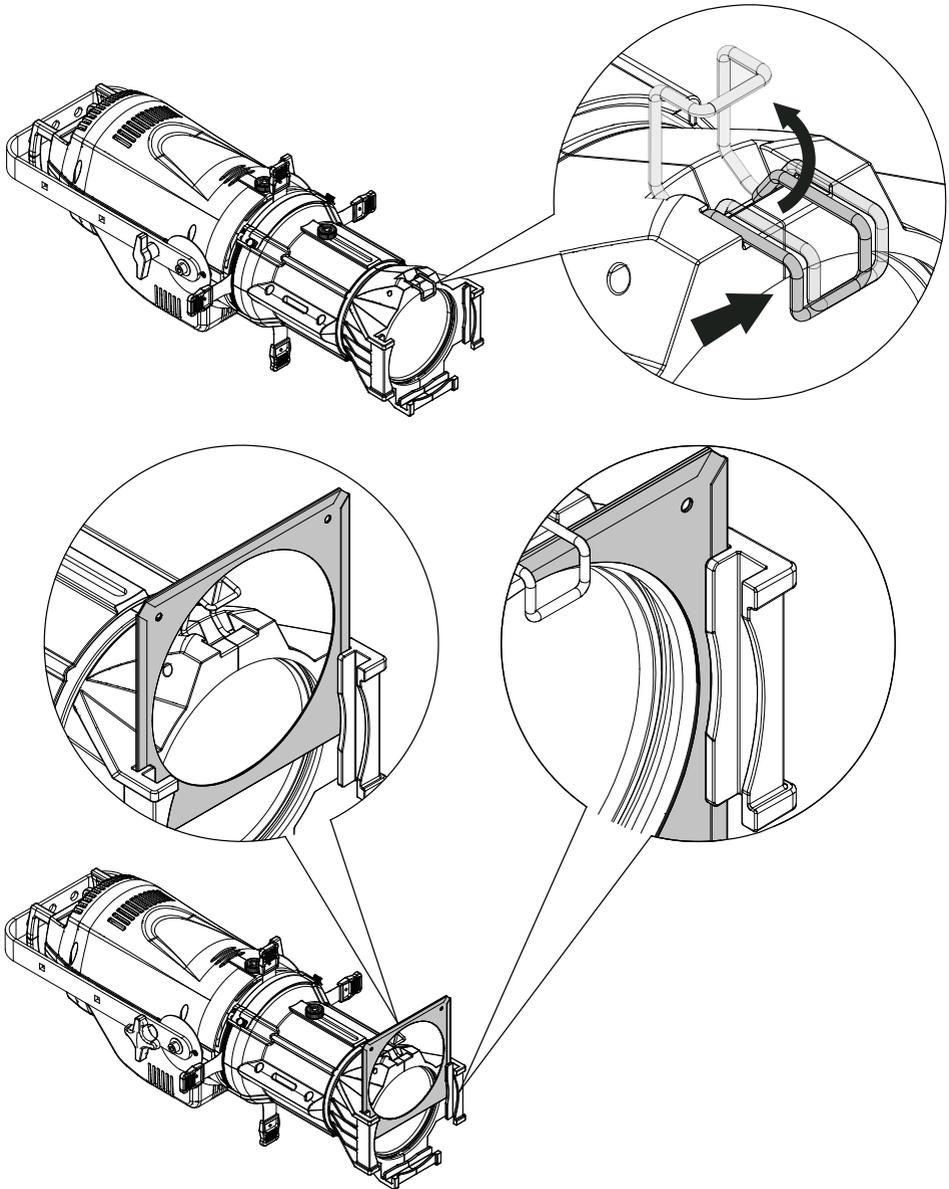
1. Push the clip, located at the top of the optics body, outwards and lift it. Then insert the filter into the marked track and close the clip, always applying an outward push.
