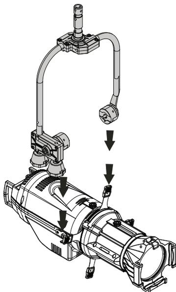
3. Mount the Pole Operated Yoke bracket.
