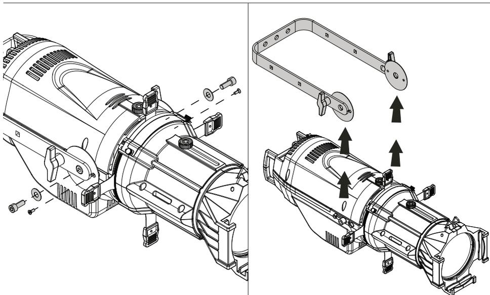
1. Loosen and remove the marked screws.
