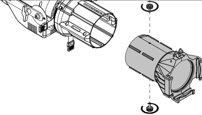
1. Loosen and remove the two marked knobs.
