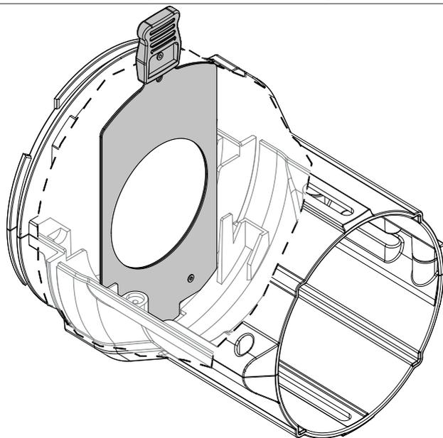
2. Insert the Soft edge filter into the slot.
