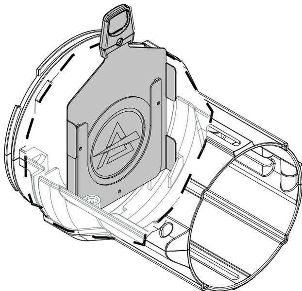
2. Insert the gobo holder into the slot. The flaps will go into the appropriate size.
