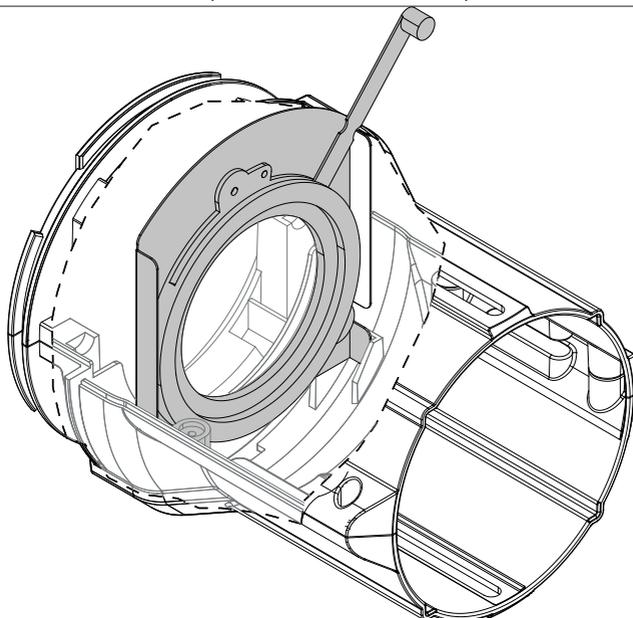
2. Insert the steel iris diaphragm into the slot. The flaps will go into the appropriate size.
