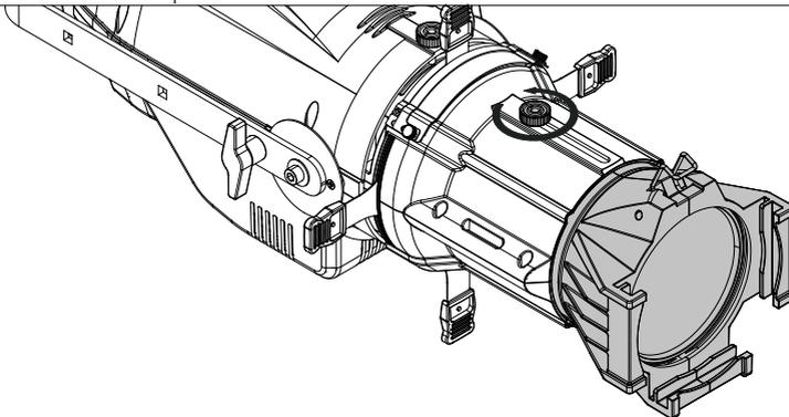
3. Insert and tighten the knobs.
