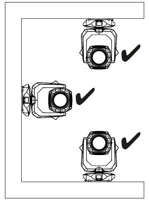
To mount the unit on a trussing system use two of the original JB-Lighting omega brackets with original Camloc-connectors. You have following four possibilities to mount the omega brackets.
