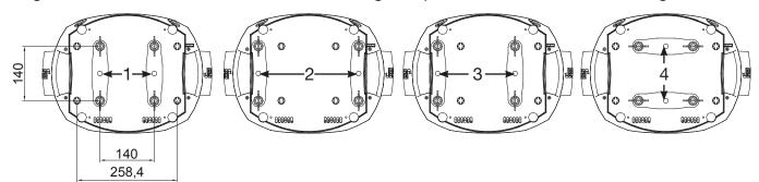
The Camlocs must snap in to be locked properly. Ensure that the structure (truss) to which you are attaching the fixture is secure. If you install the fixture to a truss always attach a safety cable, that can hold at least 10 times the weight of the fixture.
