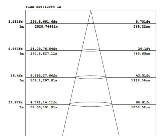
Note: The Curves indicate the illuminated area and the average illumination when the luminaire is at different distance.
