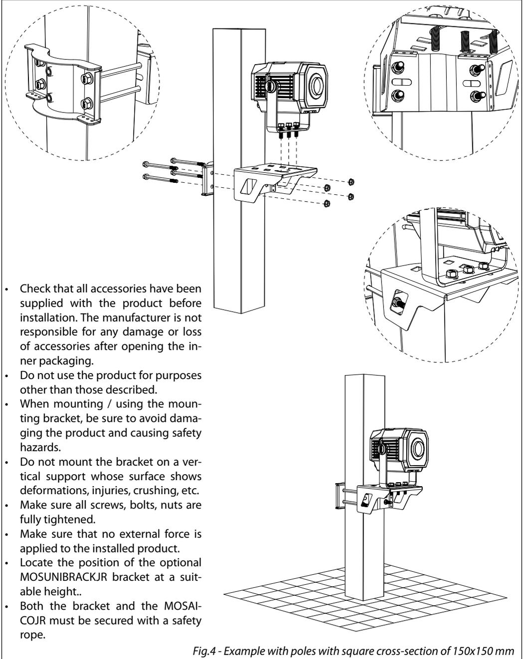
Fig.4 - Example with poles with square cross-section of 150x150 mm
