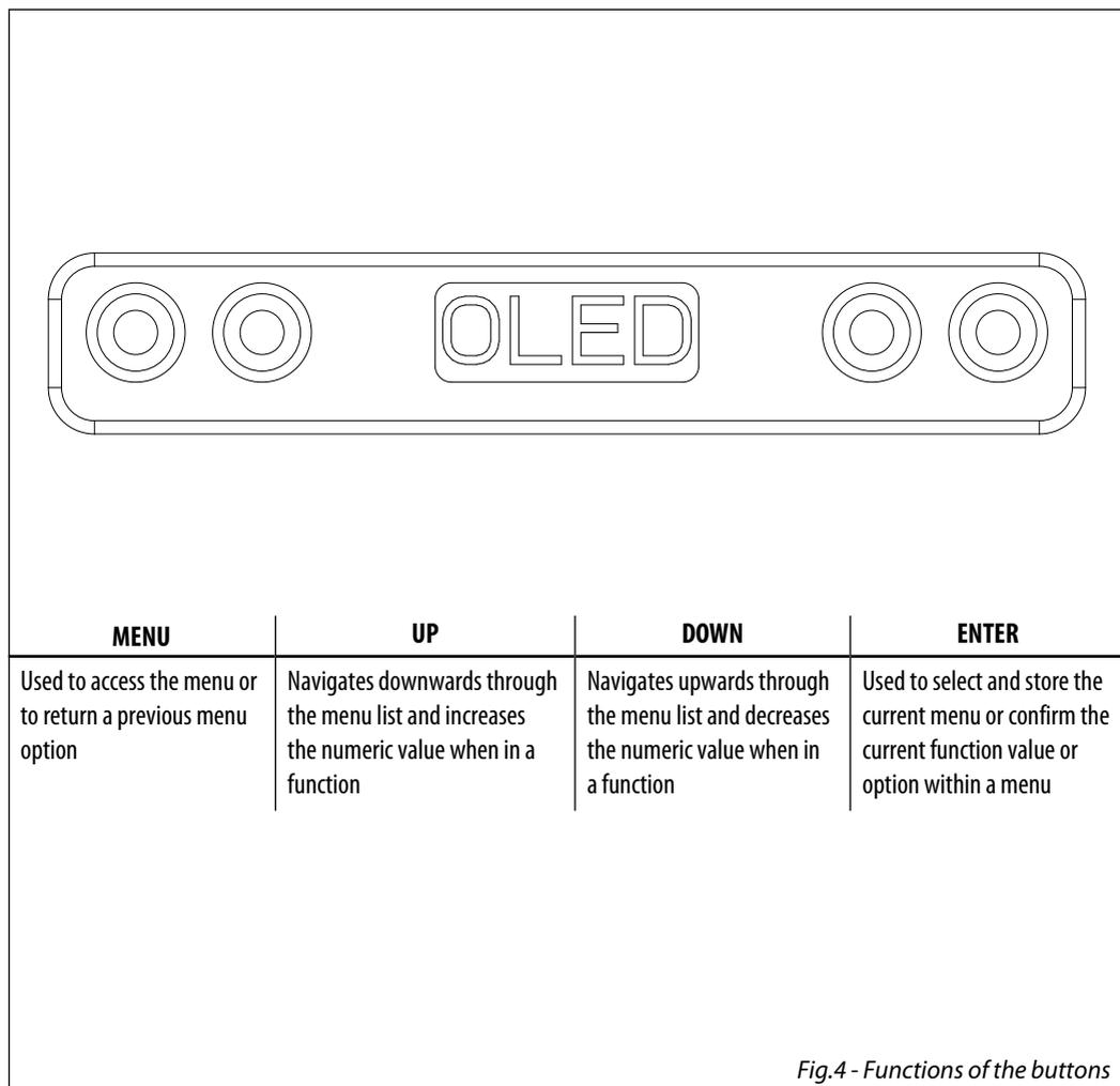
Fig.4 - Functions of the buttons
