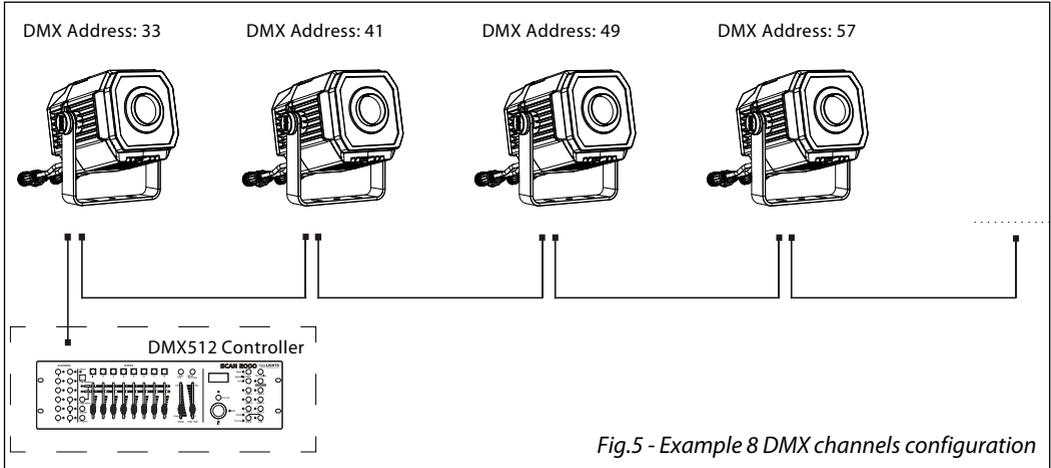
Fig.5 - Example 8 DMX channels configuration
