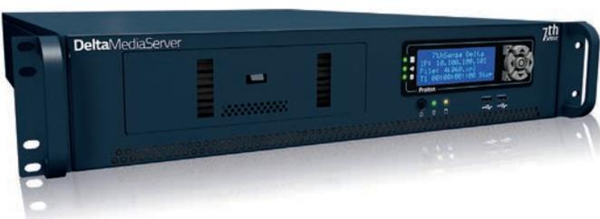
Proton comes in four different configurations and is capable of playing 4 x HD/WUXGA/2K of uncompressed playback at 60 fps in 4:4:4, or 4 x 4K 60 fps YCoCg (HAPQ).
