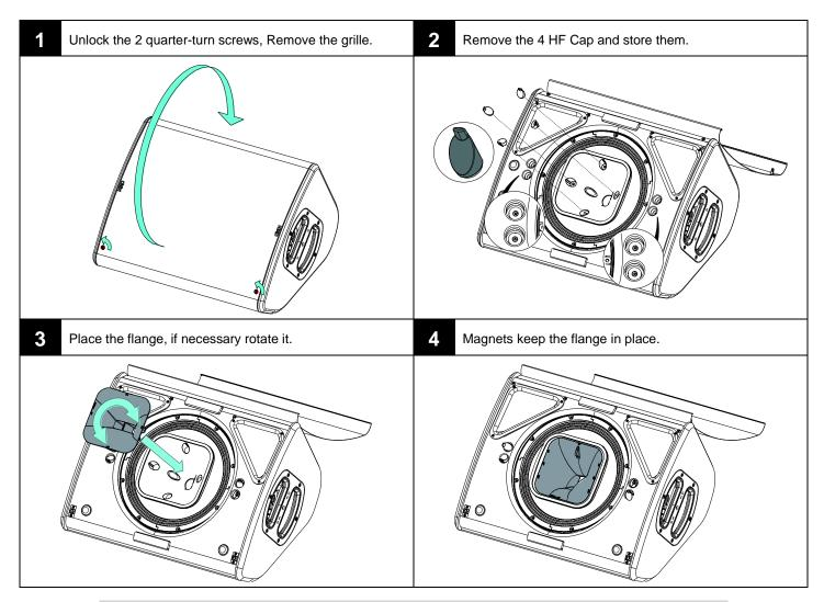
When replacing the grille, ensure it is well positioned in the top blade before fasten with quarter-turn screws.
