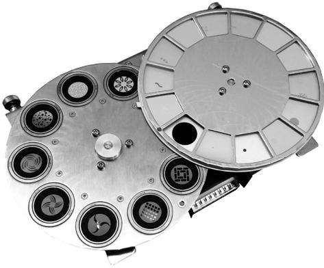
The gobos are fixed by means of a spring. To exchange a gobo pull out the spring with a pointed tool and remove the gobo out of the holder. Insert the new gobo and readjust the spring to fix the gobo. Make sure that the coated side of the glass gobo is positioned in direction of the objective.
