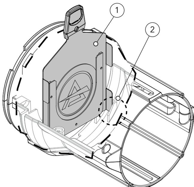
2. Insert the gobo holder (1) into the slot. The flaps will go into the appropriate size (2).
