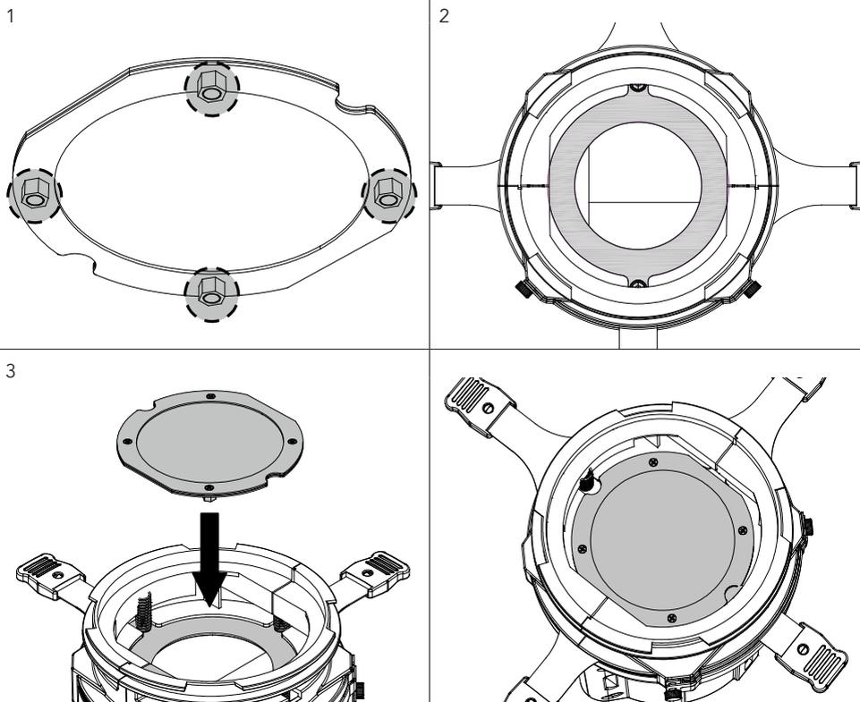
2. Insert the soft focus diffusion kit by placing the magnets (1) on the back of the framing system (2) of the middle part (3).
