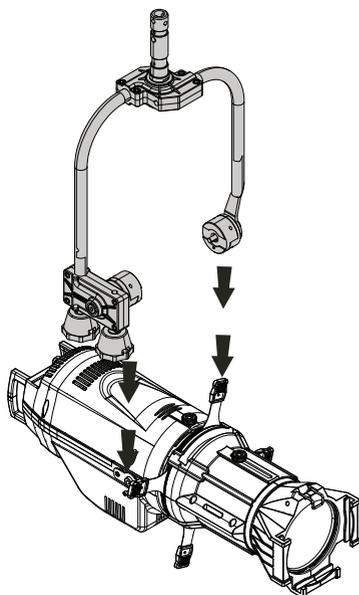
3. Mount the Pole Operated Yoke bracket.
