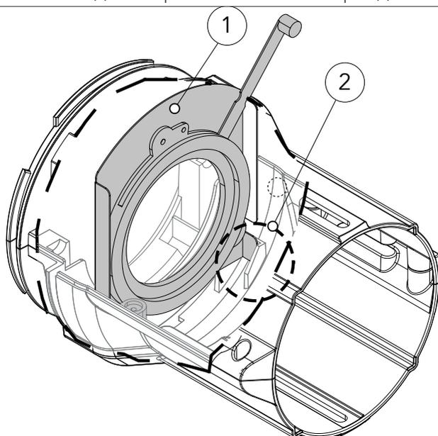
2. Insert the steel iris diaphragm (1) into the slot. The flaps will go into the appropriate size (2).
