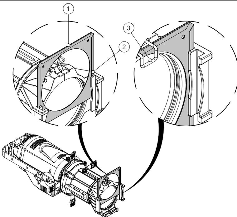
2. Then insert the filter (1) into the marked track (2) and close the clip (3), always applying an outward push.
