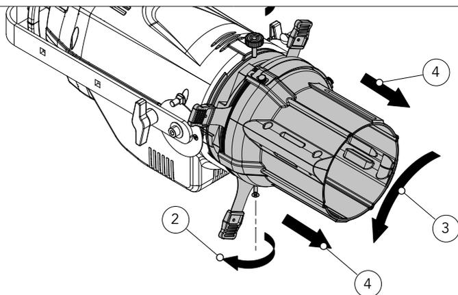
1. Loosen the marked knob (1) and screw (2). Then rotate (3) the middle part and remove it (4).
