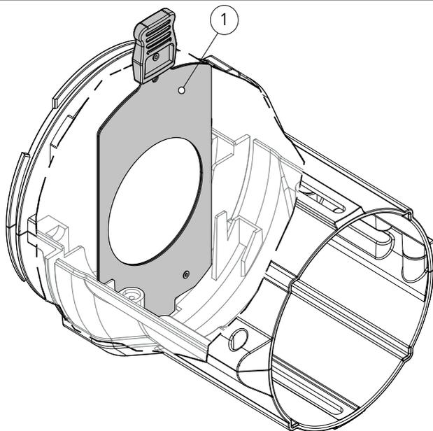
2. Insert the Soft edge filter into the slot (1).
