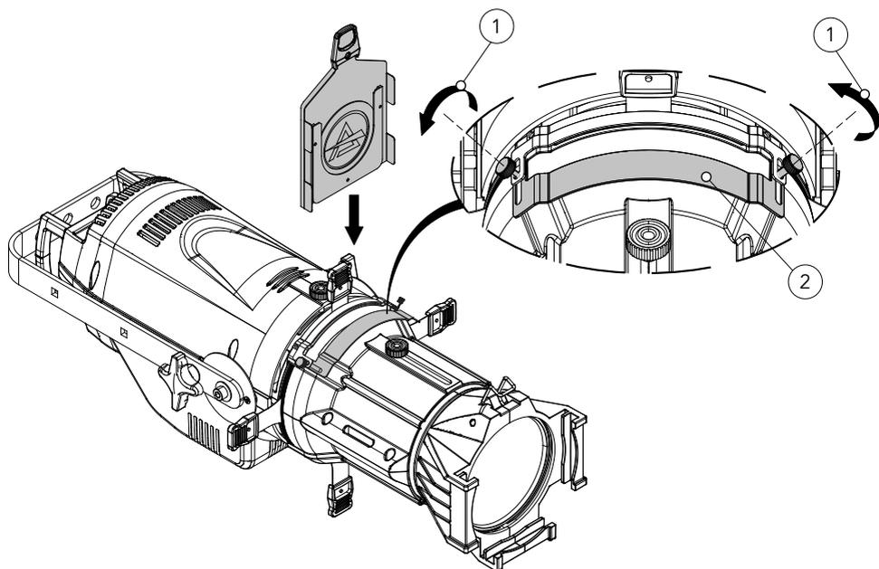
1. Loosen the marked screws (1). Then open the slot of the middle part (2).
