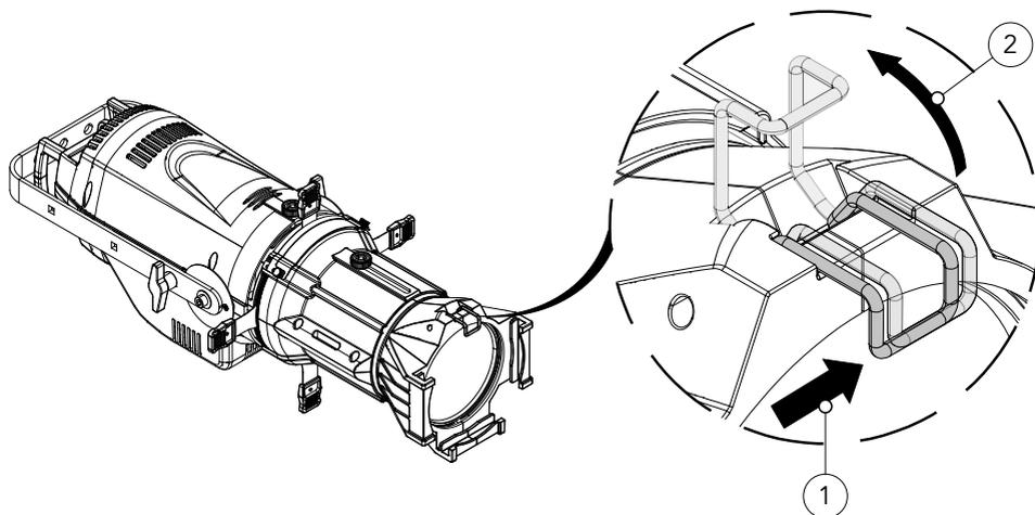
1. Push the clip, located at the top of the optics body, outwards (1) and lift it (2).
