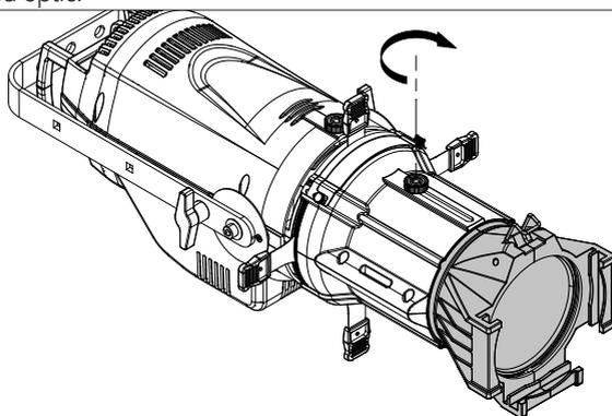
3. Insert and tighten the knobs.
