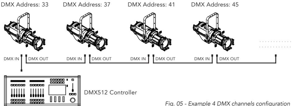
Fig. 05 - Example 4 DMX channels configuration
