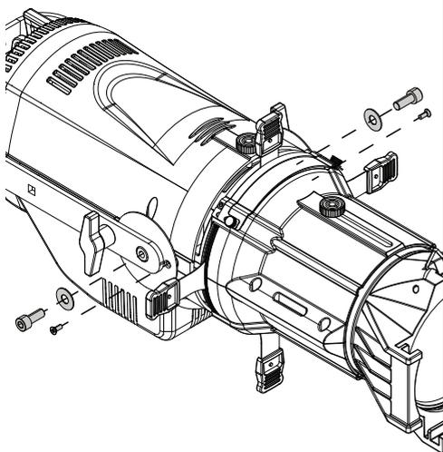
1. Loosen and remove the marked screws.
