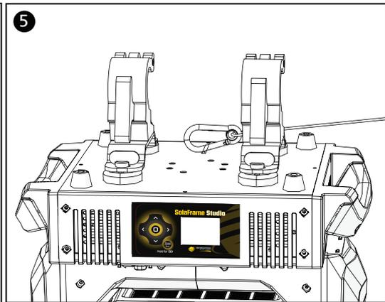
1. Assemble the clamp (provided by others) to the Omega bracket and secure together using appropriately sized hardware (not provided).
