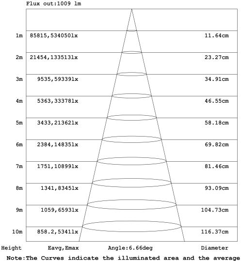
illumination when the luminaire is at different distance.
