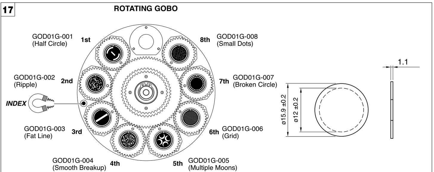
Replacing rotating gobos - Fig. 17
