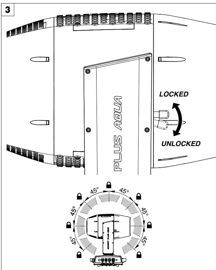
TILT Mechanism Lock and Release (every 45°) - Fig. 3
