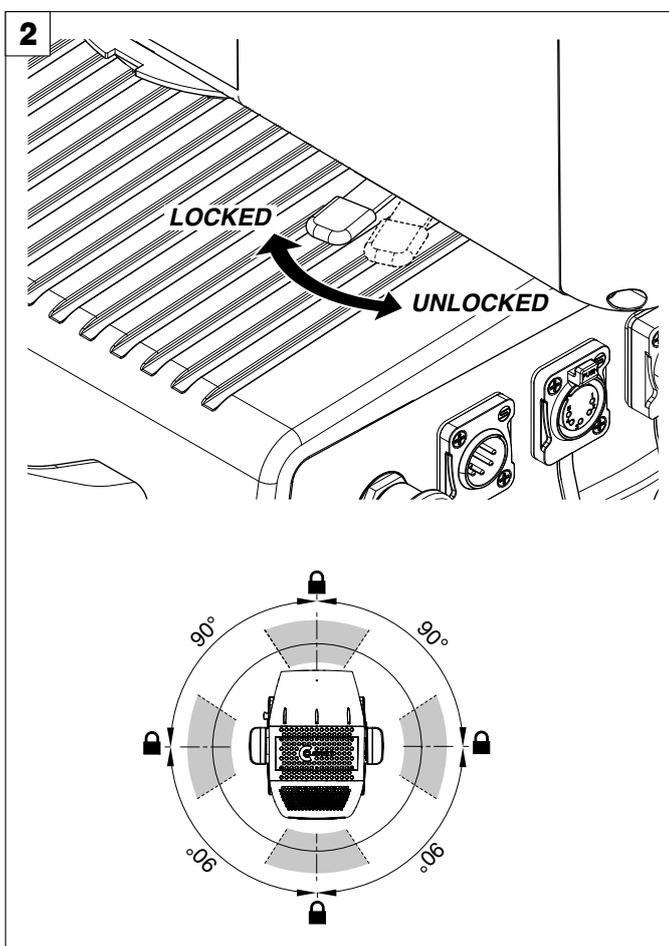
PAN Mechanism Lock and Release (every 90°) - Fig. 2
