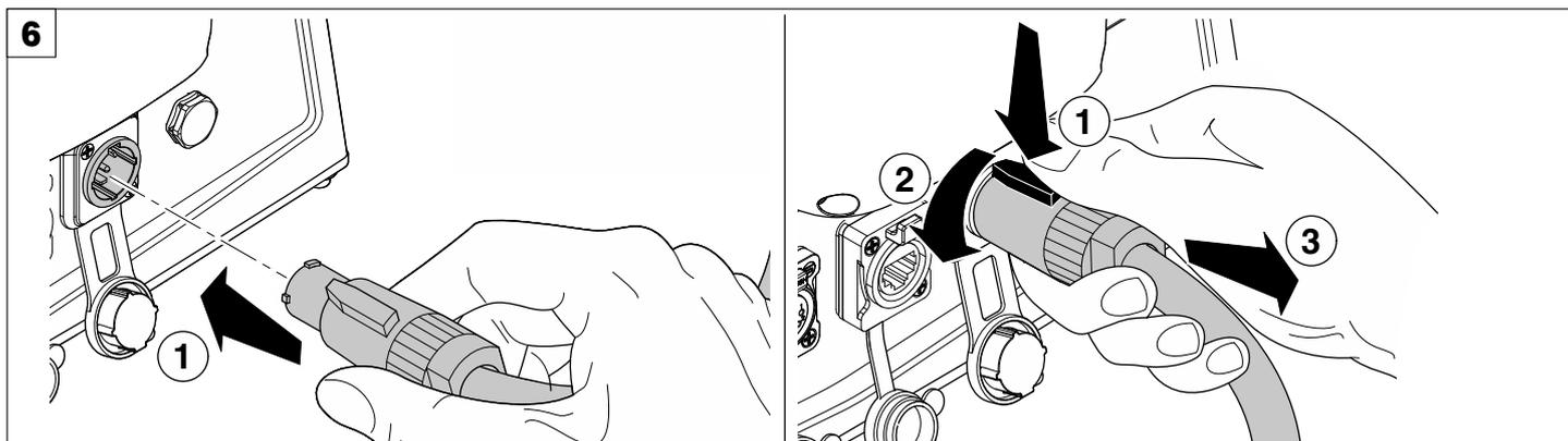
Connecting and disconnecting power cable - Fig. 6
