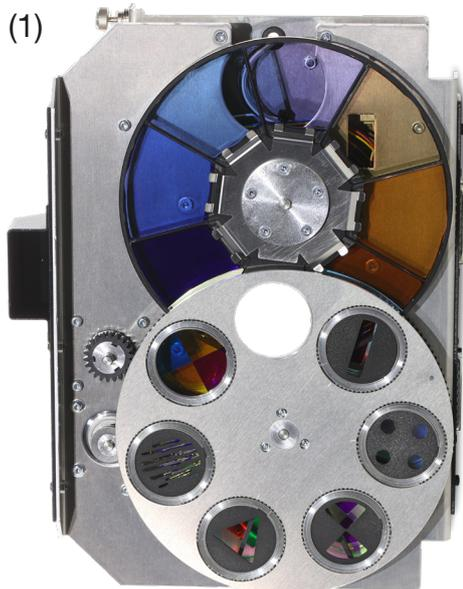
To change the gobos, remove the clamping ring A (Figure (2) - rotating gobos. Then you can replace the gobo and replace the ring. When inserting glass gobos, make sure that the coated side is facing the lens.
