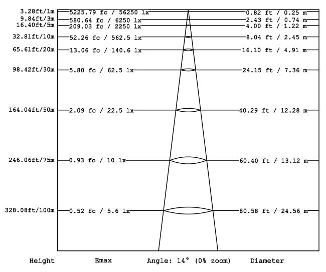
Note: The Curves indicate the illuminated area and the max illumination when the luminaire is at different distance
