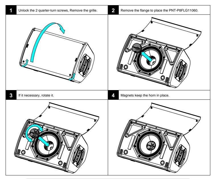
When replacing the grille, ensure it is well positioned in the top blade before fasten with quarter-turn screws.
